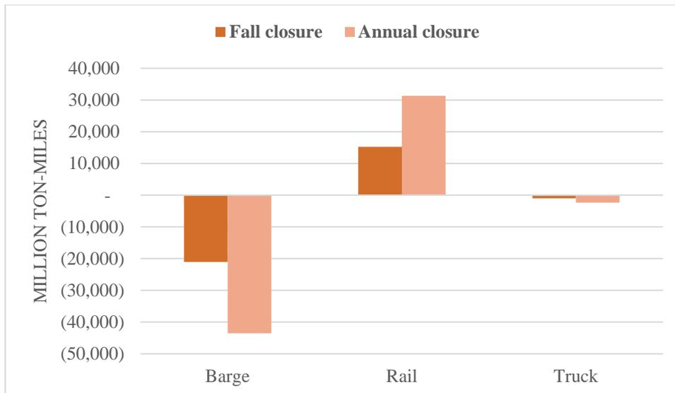
**Figure 7 Changes in mode use for corn and soybean transportation when Lock 25 is closed and rail rates remain unchanged**
